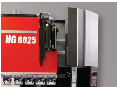
Axis movement stops when guard is opened
