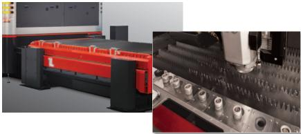
The FOL-AJ's high-speed shuttle tables and automatic nozzle changer maximize productivity. The shuttle tables externalize the material setup eliminating interference with the cutting process. The 8-station changer automatically changes, cleans and calibrates the nozzle based on material processing requirements (ensuring that the laser does not sit idle while waiting for an operator to set-up for the next job).
