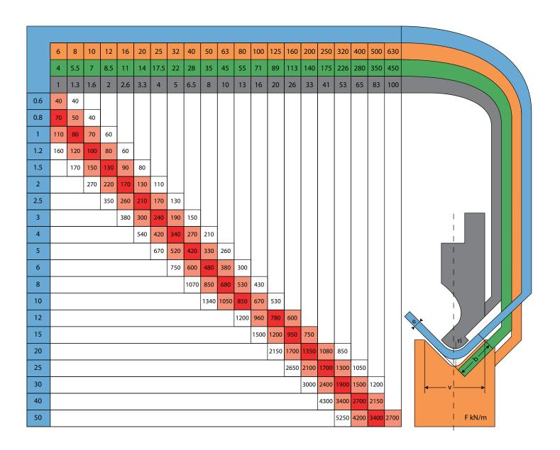
This example of an air-bending force chart is for mild-steel (40-45k/mm2 tensile strength). From the material thickness it is possible to determine:
