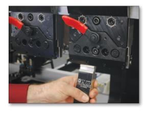
Amada's S-GRIP punch holder allows the brake operator to change punches on the press brake quickly and safely without requiring a wrench. The patented S-GRIP design dramatically decreases tool changeover time, thereby increasing bending productivity
