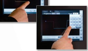
The NC control is capable of generating programs automatically. It takes into account bending constraints and ergonomics, including gauging position, component handling, bend order and required tolerance.
