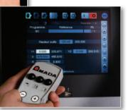
For special applications, manual mode programming allows the operator to create personalized programs.
