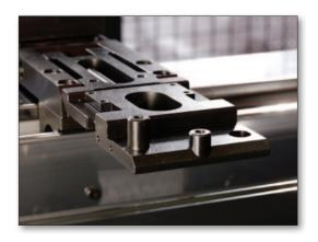
A Delta-X option is also available for the rear backstop of the 7-axis machine. This provides the stop fingers with an additional incremental adjustment of  $\pm$  6" in the X-direction. Both stop fingers can be set to different depth measurements – particularly helpful in the case of asymmetrical workpieces. Available as a single option or as a pair.
